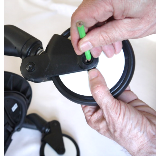
5) Insert wheel axle through first O washer
