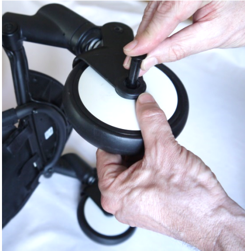
5) Insert wheel axle through first O washer
