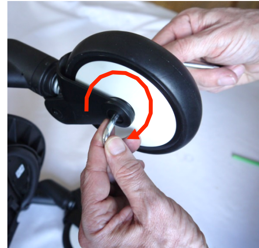
8) Using pair of L-shape tools, screw tightly
